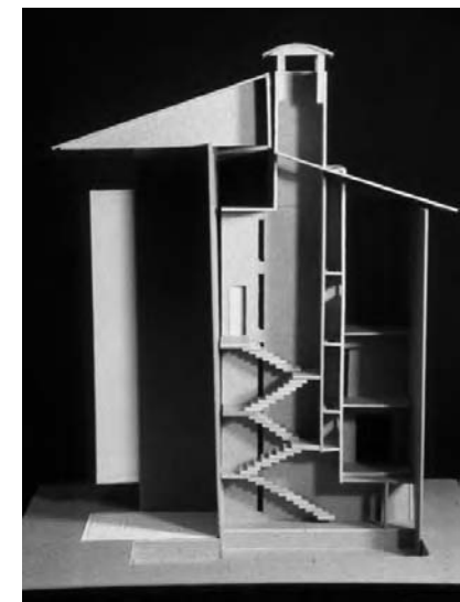
Figure 8 Beijing 12 x 12 prototype house - section model of final design, showing ventilated stair
