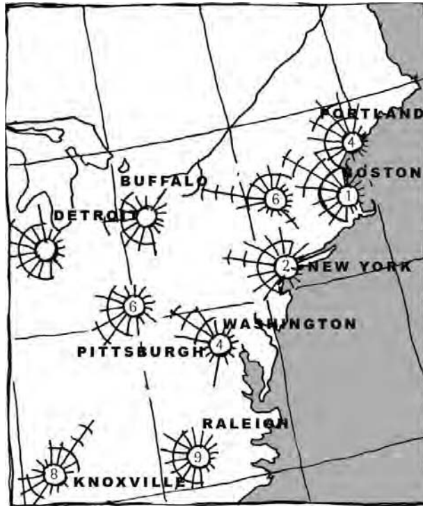
Figure 1 Surface wind roses in January for northeastern U.S. (Source: adapted from NOAA 1983)
