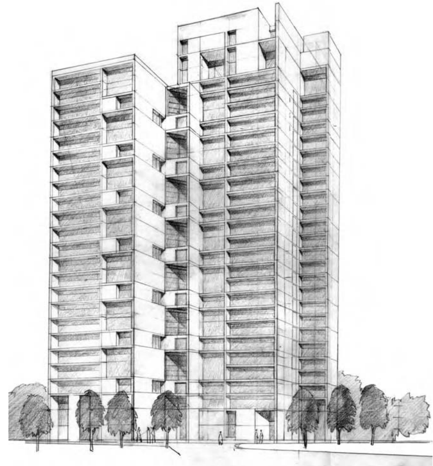
Figure 16 Perspective sketch of the final design illustrates the articulation of duplex units on the façade
