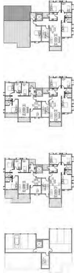
Figure 32 Plans of building I from top to bottom: top level (penthouse) floor plan, typical floor plan, ground floor plan, and basement level floor plan
