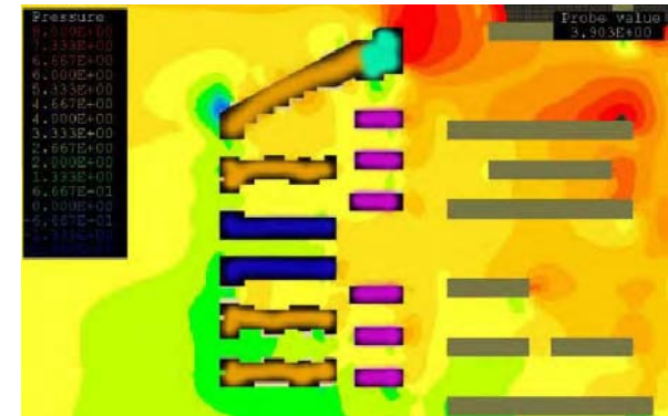
Pressure - wind from northeast
