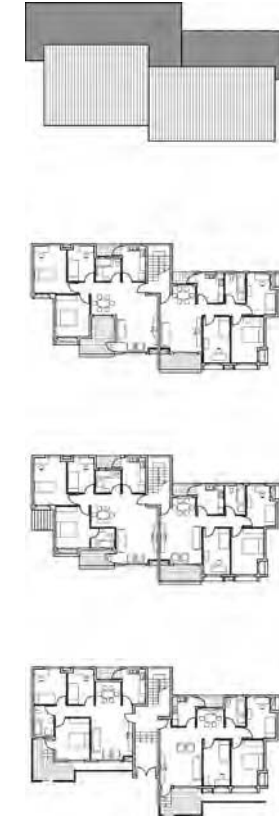
Figure 34 Plans of buildings J, K, and M (L, M, and O similar) from top to bottom: roof plan, level 4 floor plan, levels 2-3 typical floor plan, and ground floor plan
