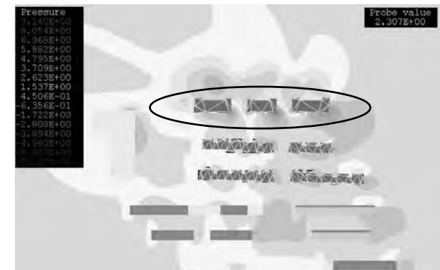
Figure 32 Images of pressure distribution around the buildings at 3 m above ground shown for: (upper) 2-building scheme, and (lower) 3-building scheme. Different gray shading levels show zones of pressure variation around building. The buildings studied are shown circled. (north is to the top in Figures 32, 33, 35, and 36)
