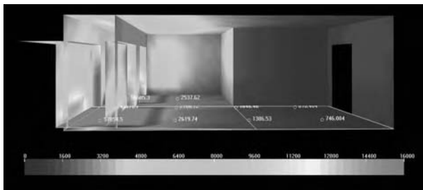
Figure 10 A false-color map of illuminance, for the same residential unit shown in Figure 9. This image gives designers quantitative information about lighting levels. (See color versions of related images in chapter 12, Figures 15-19)
